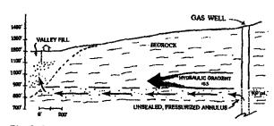
Fig. 3. An overpressured annulus located on a valley wall or upland near a valley filled with glacio-alluvial sediment may result in flow of the annulus contents laterally into valleyfill aquifers. Under the conditions depicted, the pressurized annulus has increased the normal hydraulic gradient by more than 600%.
