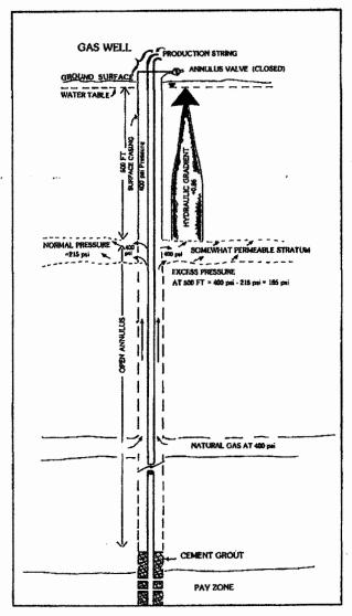
Fig. 2. Overpressuring of a well annulus by gas which is prevented from escaping to the atmosphere by a closed annulus valve. The excess pressure (185 psi) in the stratum exposed to the annulus at the 500-ft depth results in a pressure gradient of +0.86 between that stratum and the overlying water table.
